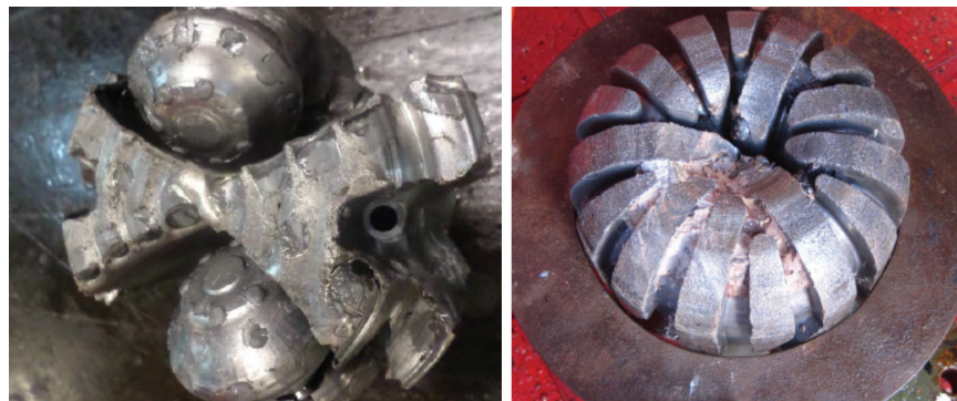
The hybrid bit design (left) with conventional rotary drilling was severely worn down at the end of its run, resulting in more bit trips and slower ROP. The TurboForce™ diamond-impregnated bit design (right), used with the Turbopower™ turbodrill, was in excellent condition at the end of its run, thus improving drilling length intervals and ROP.
