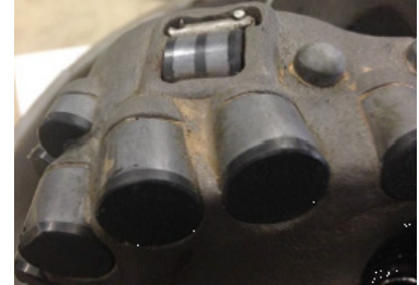
Shows condition of bit following operator's record run (4.9 hour curve)
