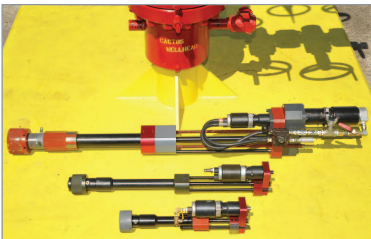
Hot tap units are available in 20-in. unit, 13-in. unit and 7-in. stroke sizes.
