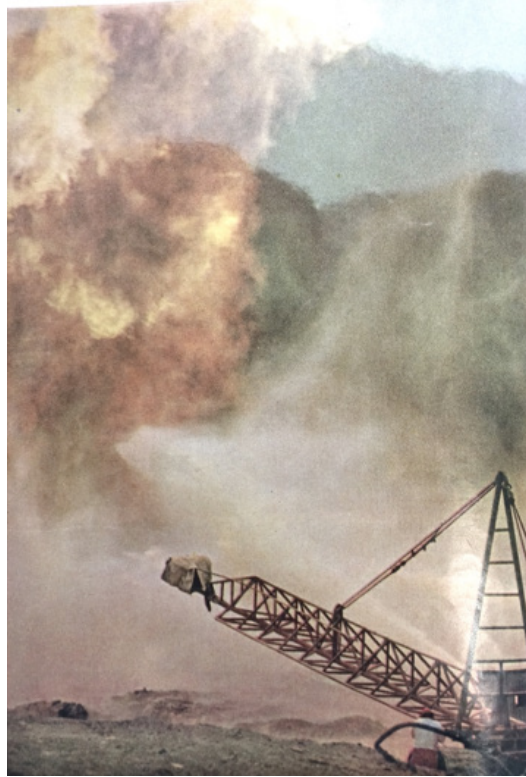
Figure 3. Athey wagon with 1,100 pounds of explosives. Courtesy of R. Hatteberg and LIFE Magazine.
