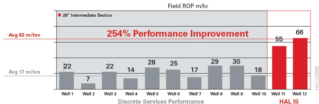
Graph showing ROP performance improvement in 28-in riserless section of the Halliburton IS project, over that of previous wells in the field
