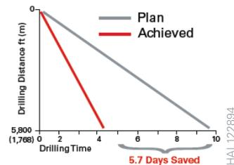
Graph showing Drilling Times in 16-inch Salt section
