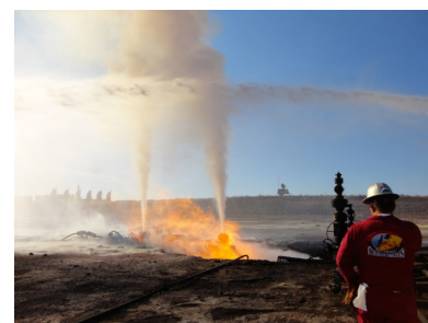
Figure 2. The fires of three proximate wells feed each other to create a complex fire hazard on the site. The side valve of the well on the right is compromised and is feeding a mixture of gas and condensate to the other two wells.
