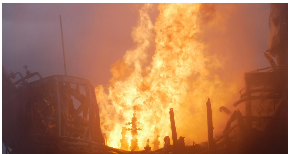
Fire erupts on an offshore production platform in the Caspian Sea, where an explosion in a gas pipeline caused a fire that triggered multiple wells to develop leaks and blowouts.
