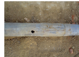
The snubbing unit found multiple instances of corrosion damage in the production tubing that it recovered.
