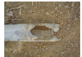
The snubbing unit found multiple instances of corrosion damage in the production tubing that it recovered.
