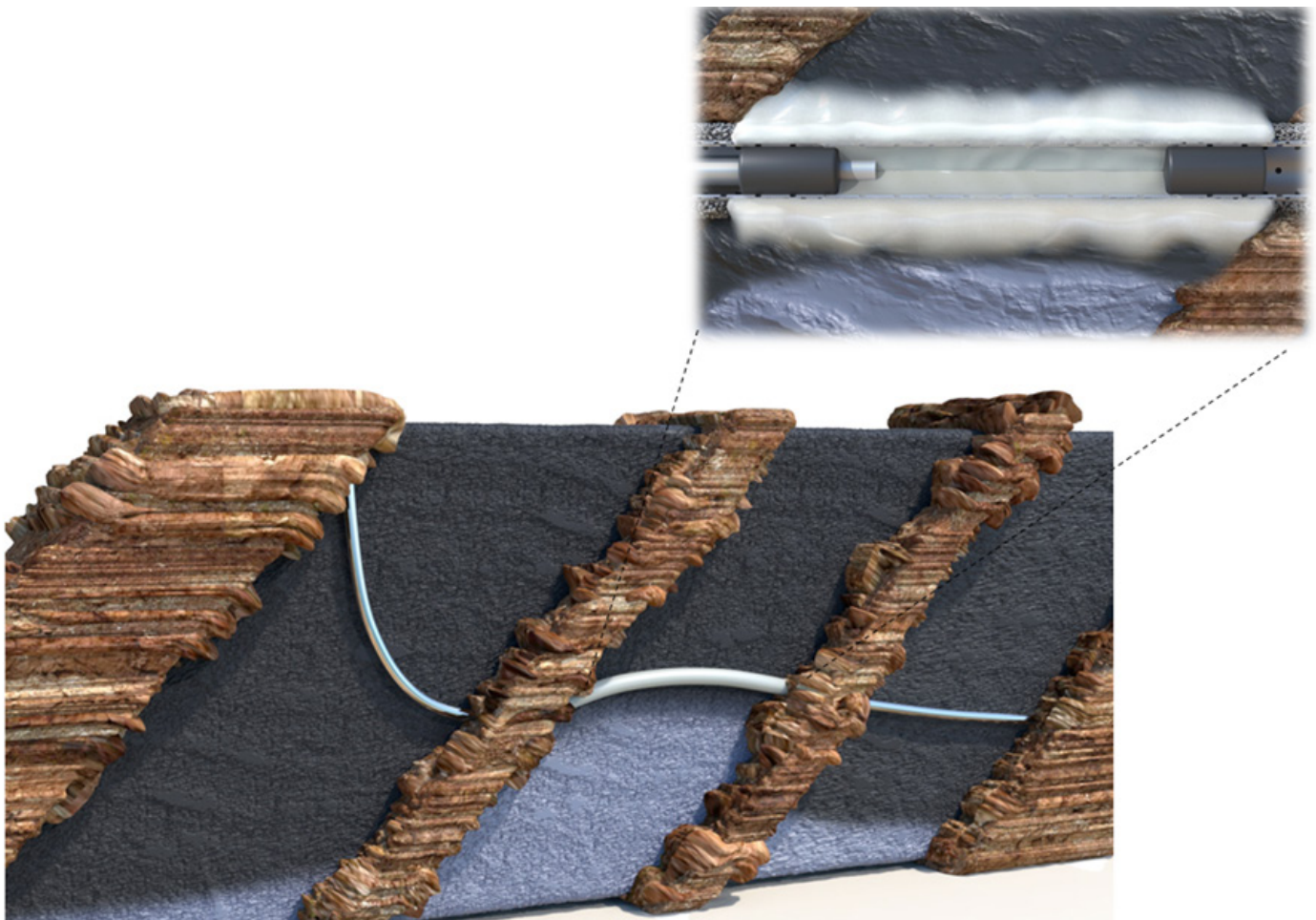
EquiSeal™ Conformance application > Conformance treatment is placed with the aid of coiled-tubing and using packers to mechanically isolate the targeted area. EquiSeal™ optimum viscosity profile allows for an accurate placement of the treatment into the targeted zone.
