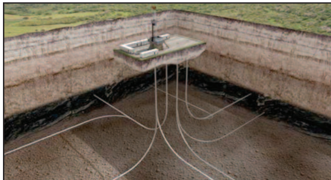
Single Pad with Four Dual-Lateral Horizontal Wells (Eight Wellbores)
