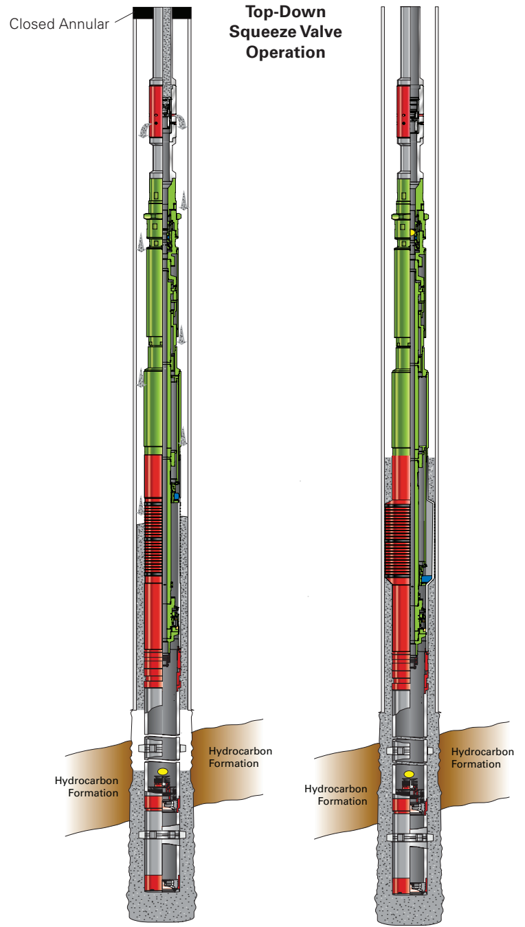
Top-Down Squeeze Valve Opened and Job Performed
