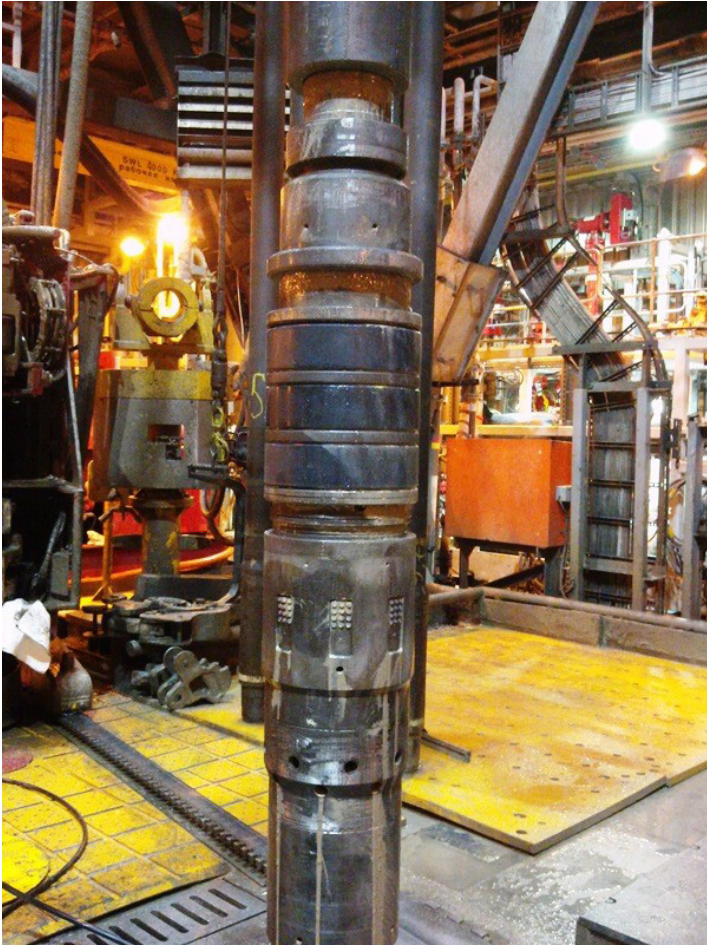
A 13 3/8-in. Inflow Tech® packer is pulled out of hole.
