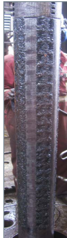
PowerMag® magnets with over 250 lb of debris
