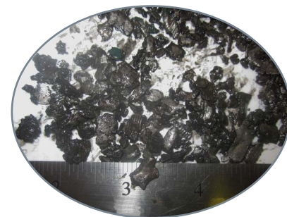
Perforation debris collected by PowerMag® magnets
