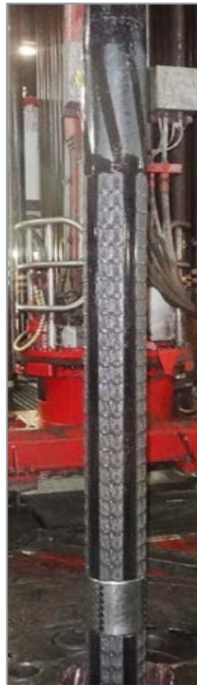
PowerMag® magnet from Assembly 1: 116.5 lb of metal fines
