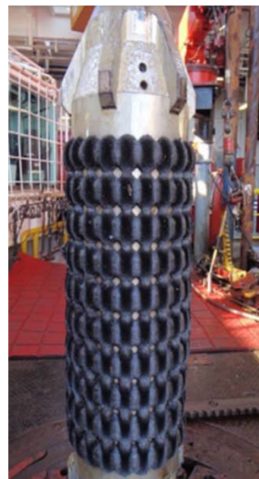
Well #2 Riser Mag Tech® riser magnet with 14.23 kg of fine metal shavings
