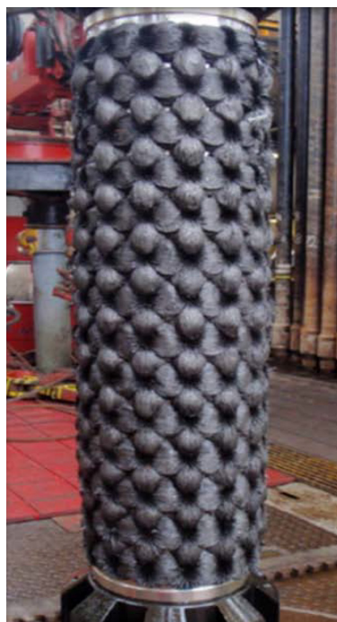
Well #1 13 5/8-in. Mag Tech® casing magnet with 25.03 kg of fine metal shavings
