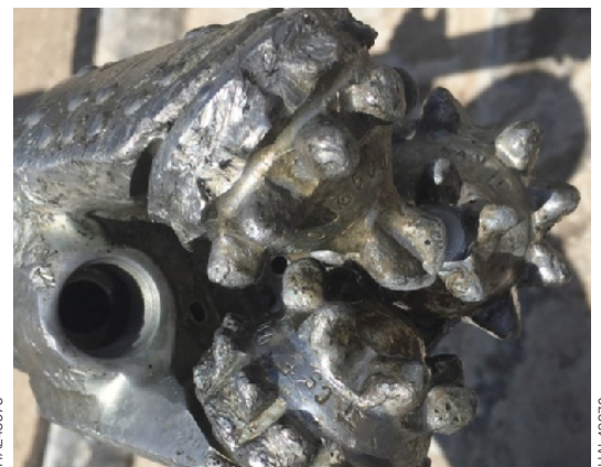
Roller cone Bit #2 - Drilled out 54 Obsidian® frac plugs with one short-trip after 30 Obsidian plugs
