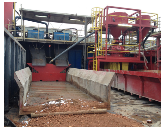
BaraG-Force™ VacVCD with cuttings collection trough inside a three sided catch tank.
