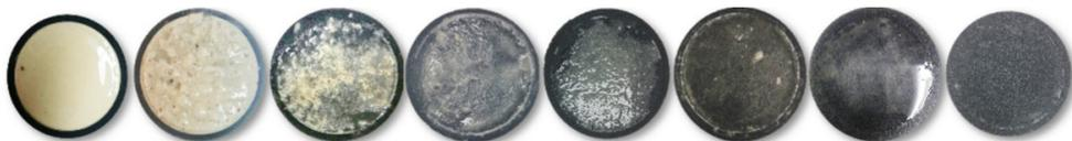
Lab tests using ceramic disks show filter cake accumulation before and after treatment with the N-FLOW™ 325 system. In the Boscán field, 12–14 hours of soaking time are required for the in-situ acid to dissolve the filter cake, based on lab testing and field observations.
