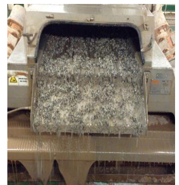
Figure 1 PERFORMADRIL® system helps preserve cuttings integrity and improve solids control efficiency.
