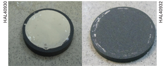
Lab tests showing filter cake on ceramic disks, before (left) and after (right) N-FLOW™ 325 breaker treatment.
