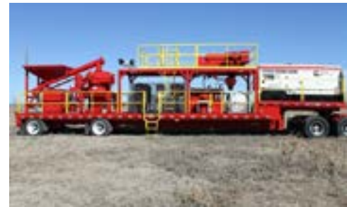
The Baroid Mobile VCD/Centrifuge combination is easy to rig up and operate at any onshore rigsite.
