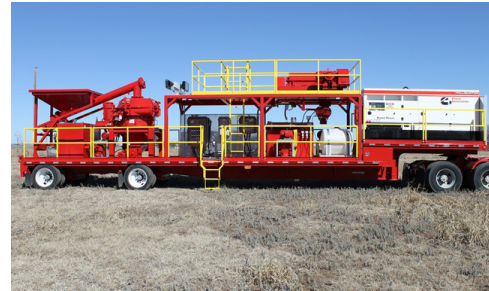
The Baroid Surface Solutions Mobile VCD/ Centrifuge combination is easy to rig up and operate at any onshore rigsite.
