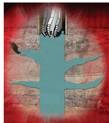
The complexity of curing lost circulation depends on the formation type and the rate of fluid loss.
