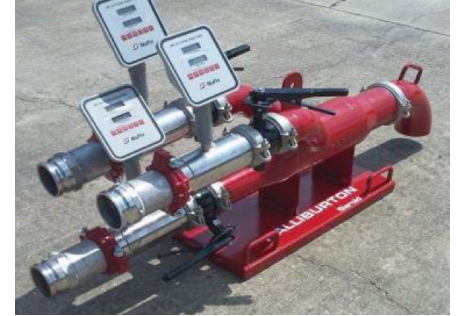
Figure 1 Mix On The Fly (MOTF) unit
