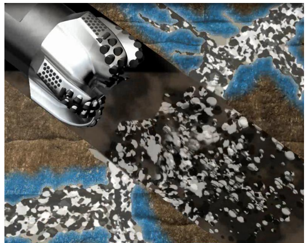
HYDRO-PLUG™ lost circulation material – Superior Fracture Sealing Performance
