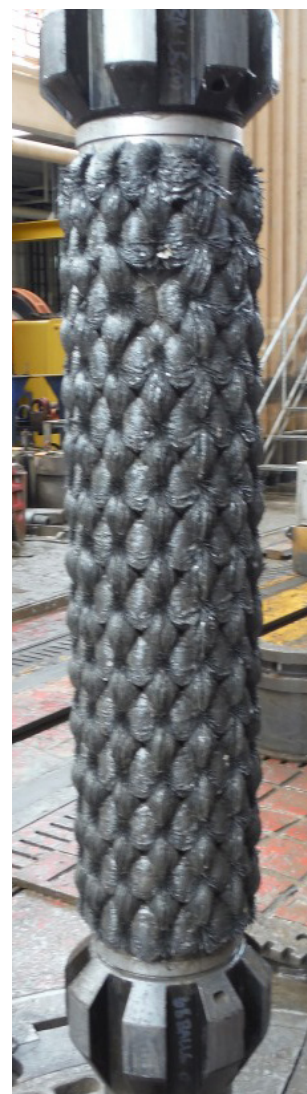
This magnet scraper is water-wet and residue-free after application of BaraKlean®-648 casing cleaner.
