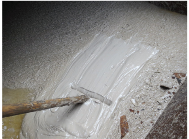
Wellbore cleanup failure: Initial third-party wellbore cleanup failed to remove contaminated OBM residue due to a lack of planning.
