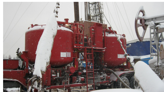
Halliburton batch mixer used to mix LCM pill
