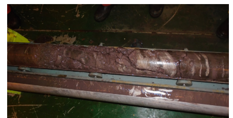
This highly fractured carbonate formation is prone to severe lost circulation.
