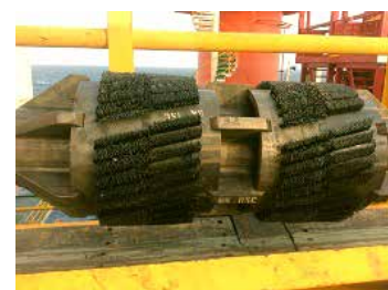
This brush is residue-free after application of an engineered cleanout spacer containing BaraKlean®-648 casing cleaner.
