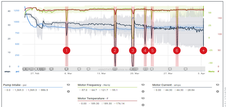
Field tests show continuous restarts with low stress on the ESP.
