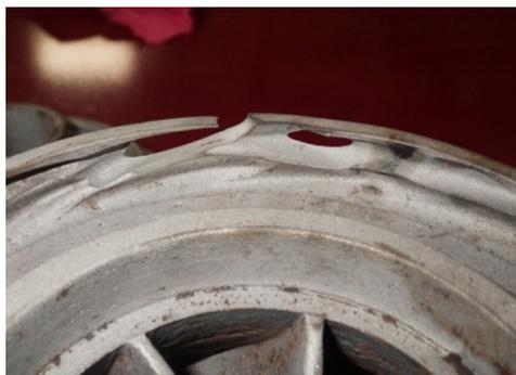
Left » Erosion was significant in standard style diffusers.
