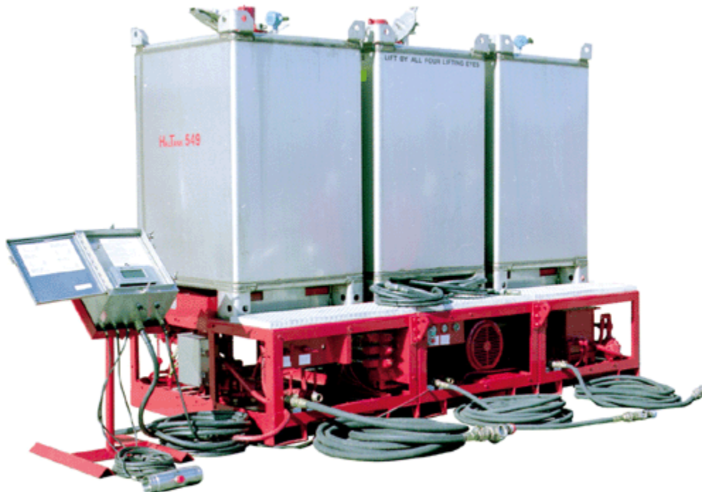
Figure 4: Mobile control center that allows customers to observe cementing parameters in real-time
