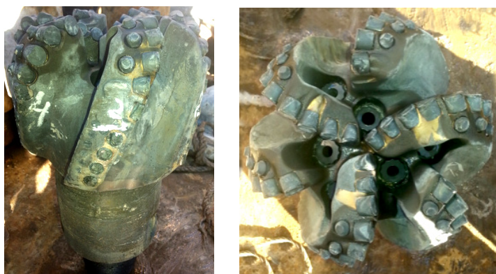
Drill bit comparison. The retrieved drill bit showed only minor signs of wear.
