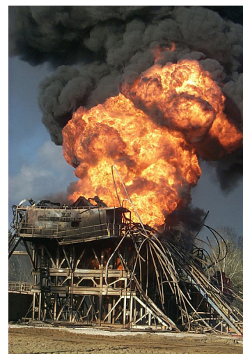
After a blowout, the damaged drilling rig is on fire.
