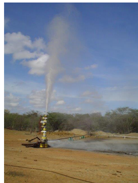
Prior to Boots & Coots regaining control of this well, gas flows in full open mode through the crown valve and a hole in the wellhead.
