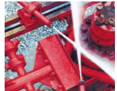
Figure 4. The Halliburton abrasive jet cutter can reduce readying a new wellhead from 30 hours to 30 minutes, and this innovative tool contributed in large measure to the success of the Boots & Coots operation in Kuwait. (Photo courtesy of R. Hatteberg)
