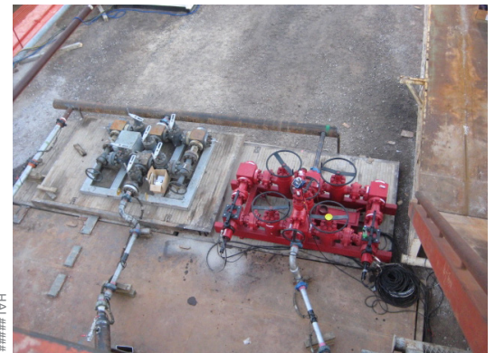
Choke Manifolds: Manual (left) and Hydraulic (right)
