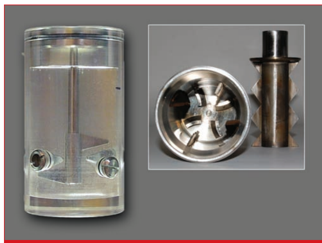
Figure 7 – The patented Mimic device components are designed to work with a conventional viscometer. The Mimic device enables measurement of the elastic transport properties of a viscoelastic fluid.
