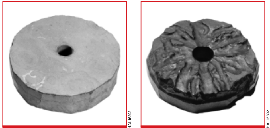
Figure 1—The left-side sample is a limestone (calcite) core as it was taken. On the right is a view of the same core showing the uneven etching that is the goal of a Carbonate 20/20 treatment. A formation etched in this manner will resist crushing from overburden pressure.
