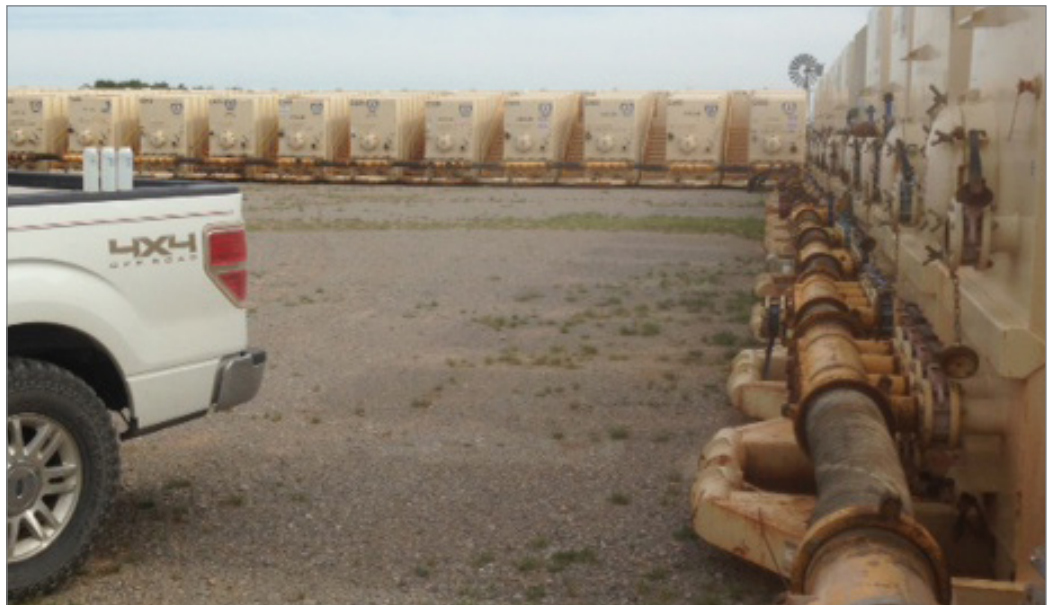
With a cost-effective biocide, Multi-Chem successfully treated 31 frac tanks that were contaminated with acid producing bacteria, saving the operator 650,000 gallons of water.
