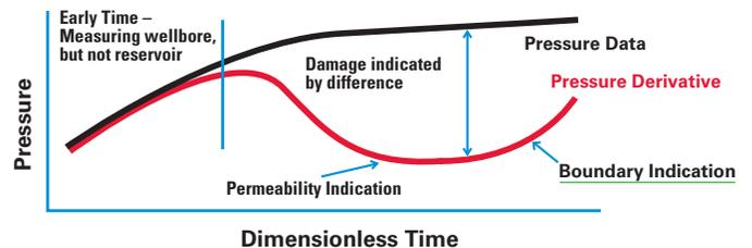
Mini drillstem testing example
