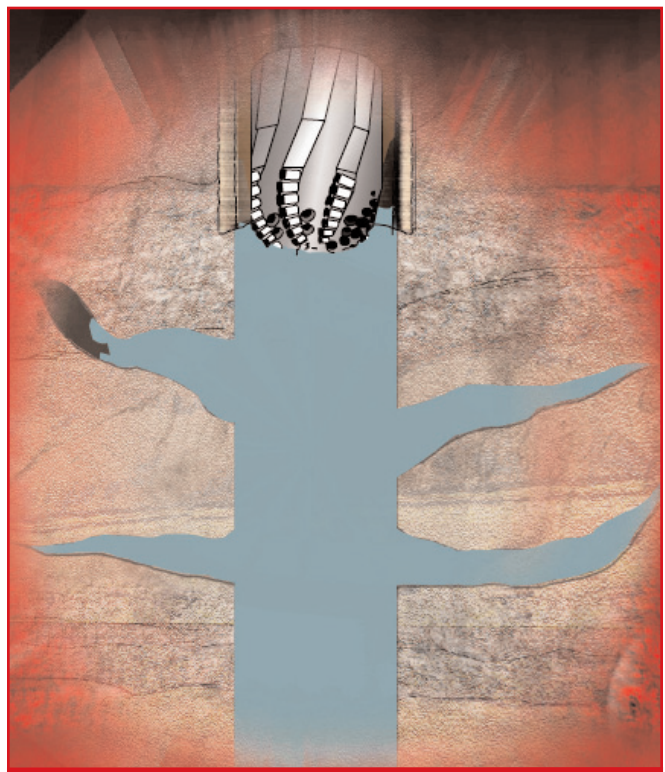
FUSE-IT™ lost circulation material can be squeezed into loss zones to seal fractures.
