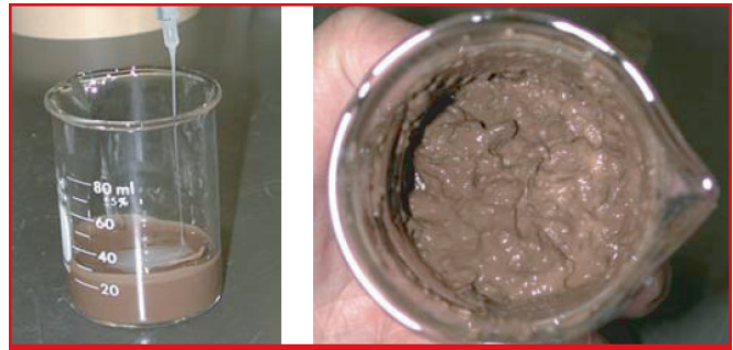
FUSE-IT system added to lignosulfonate mud sample in a 1:20 ratio.
